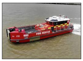
allow crews to fight fires from the river as well as a hydraulic crane and thermal imaging camera that can be used to carry out rescues from the water. They will provide a significantly improved mass rescue capability with each boat capable of carrying up to 45 people.
